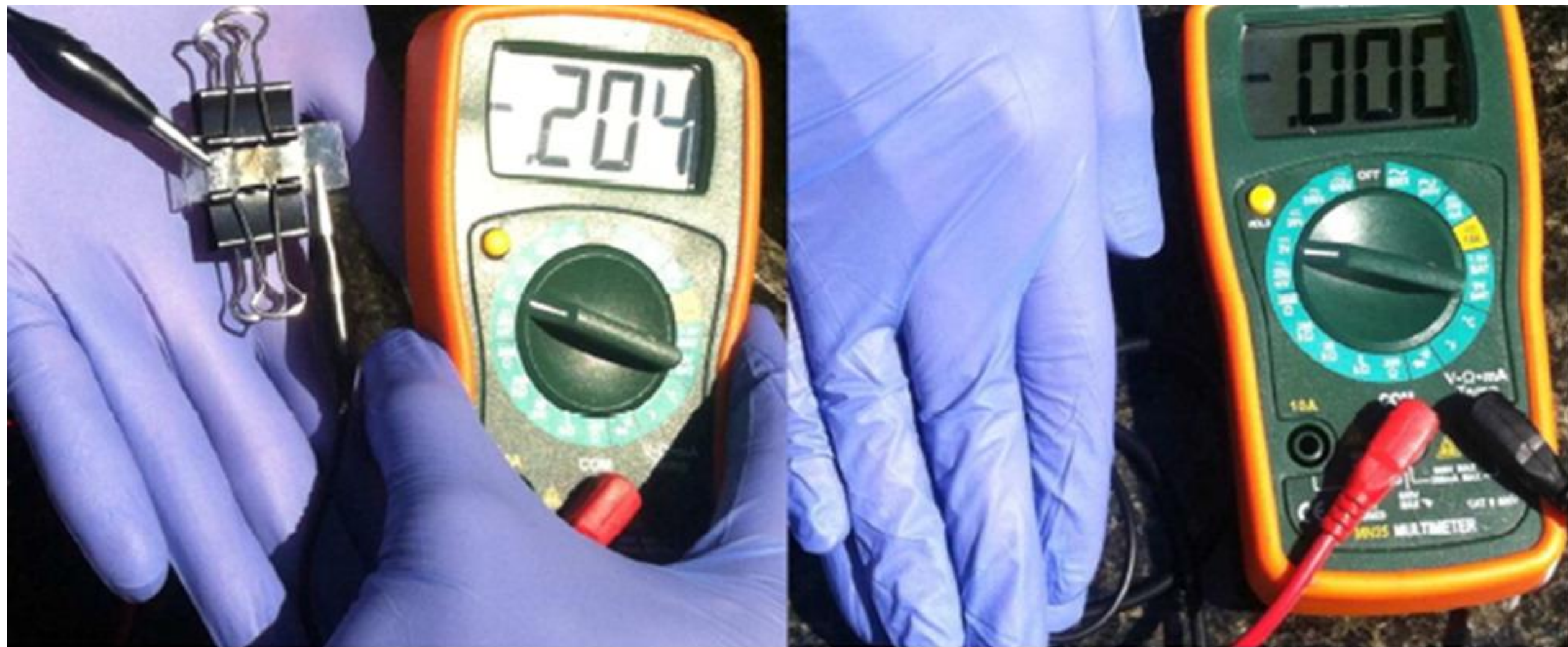
Measurement of the photovoltage under sunlight and in dark conditions. The device is kept in the palm of one hand, controlling the exposure to sunlight with the other.
